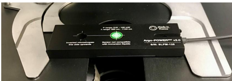
Figure 20: Argo-POWER HM head inserted in the sample holder of an inverted microscope; the target, on the opposite side of the sensor, is illuminated with the white light coming out from the condenser.
