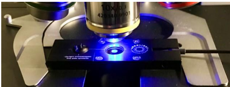
Figure 19: Argo-POWER HM head inserted in the sample holder of an upright microscope; the sensor is illuminated with blue light, at its center.
