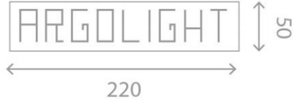
Figure 18: Schematics of the word ARGOLIGHT. All dimensions are in \mu\text{m} .
