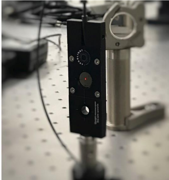
Figure 21: Argo-POWER HM head inserted across the optical path of a collimated light beam.
