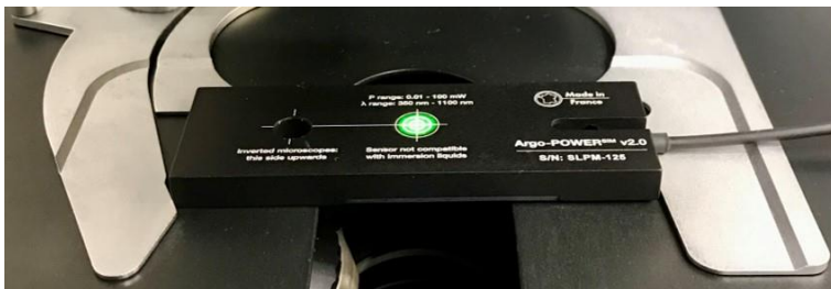
Figure 15: Argo-POWER LM head inserted in the sample holder of an inverted microscope; the target, on the opposite side of the sensor, is illuminated with the white light coming out from the condenser.
