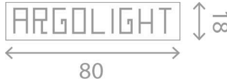
Figure 18: Schematics of the word ARGOLIGHT. All dimensions are in \mu\text{m} .
